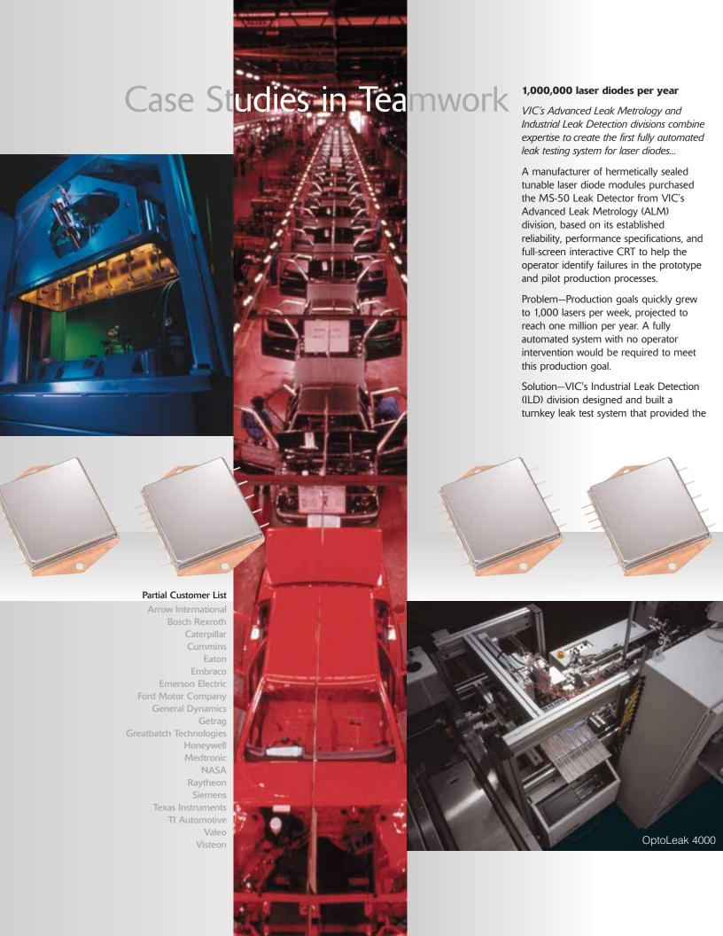
most efficient solution: The new OptoLeak 4000 is the first fully automatic leak detection system to offer magazine-to-magazine testing of devices in standard Auer® boat carriers. The OptoLeak 4000 employs the MS-40 leak detector for accurate testing, and bar code scanning for complete data acquisition.
